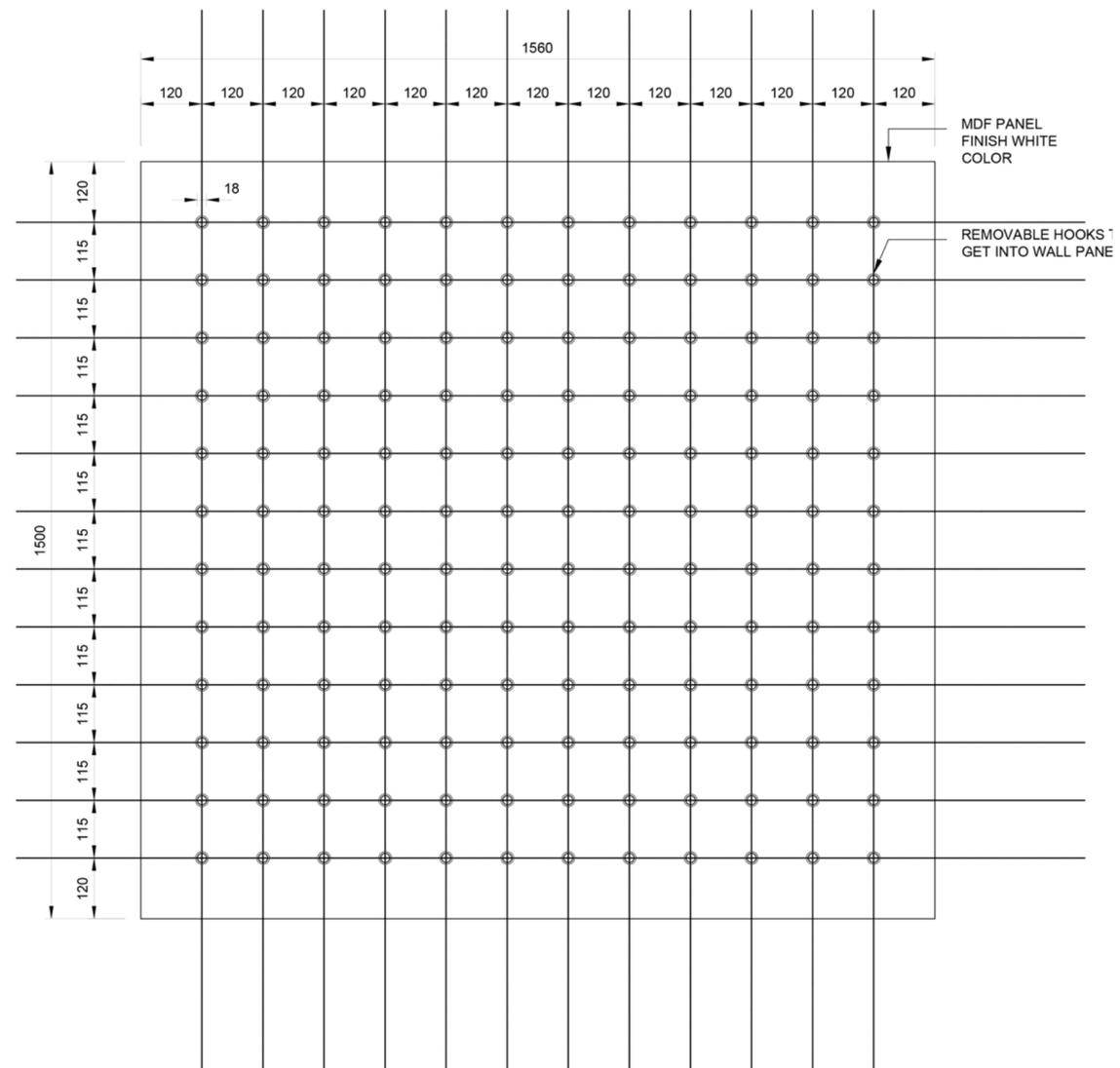
Structural Front Elevation Display (Detail 1302-03 C)
